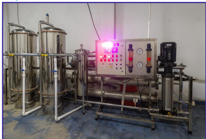
6000 LPH SS RO Plant
